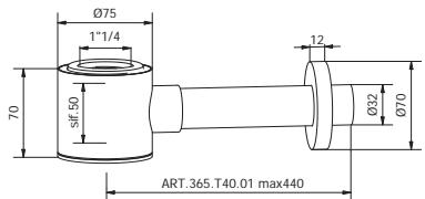
SIFONE SALVASPAZIO KOMPATTO PER LAVABO - FILETTO PER PILETTA 1"1/4, CON SCARICO ORIZZONTALE TUBO SCARICO 300 mm
