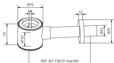
SIFONE KOMPATTO UNIVERSAL PER LAVABO - FILETTO CENTRALE PER PILETTA UNIVERSAL, CON SCARICO ORIZZONTALE, TUBO SCARICO 300 mm
